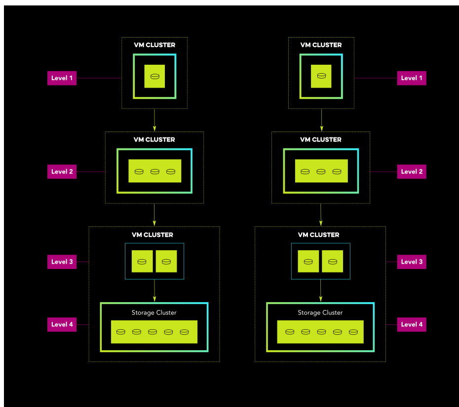
Figure 29: Example query execution tree that shows four levels of multiple clusters
